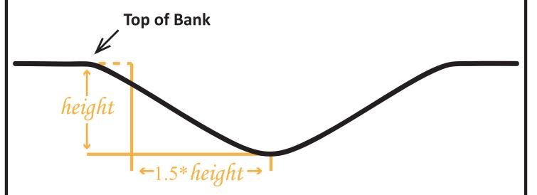
Case where existing slope of the bank is less steep than 1.5 (horizontal): 1 (vertical)
