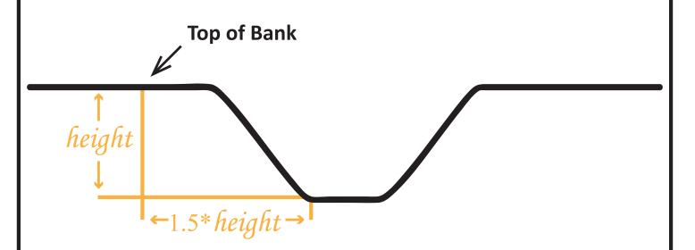
Case where existing slope of the bank is steeper than 1.5 (horizontal) : 1 (vertical)
