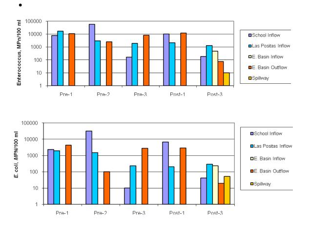
Figure 3. Fecal indicator bacteria concentrations on East side of Project.
