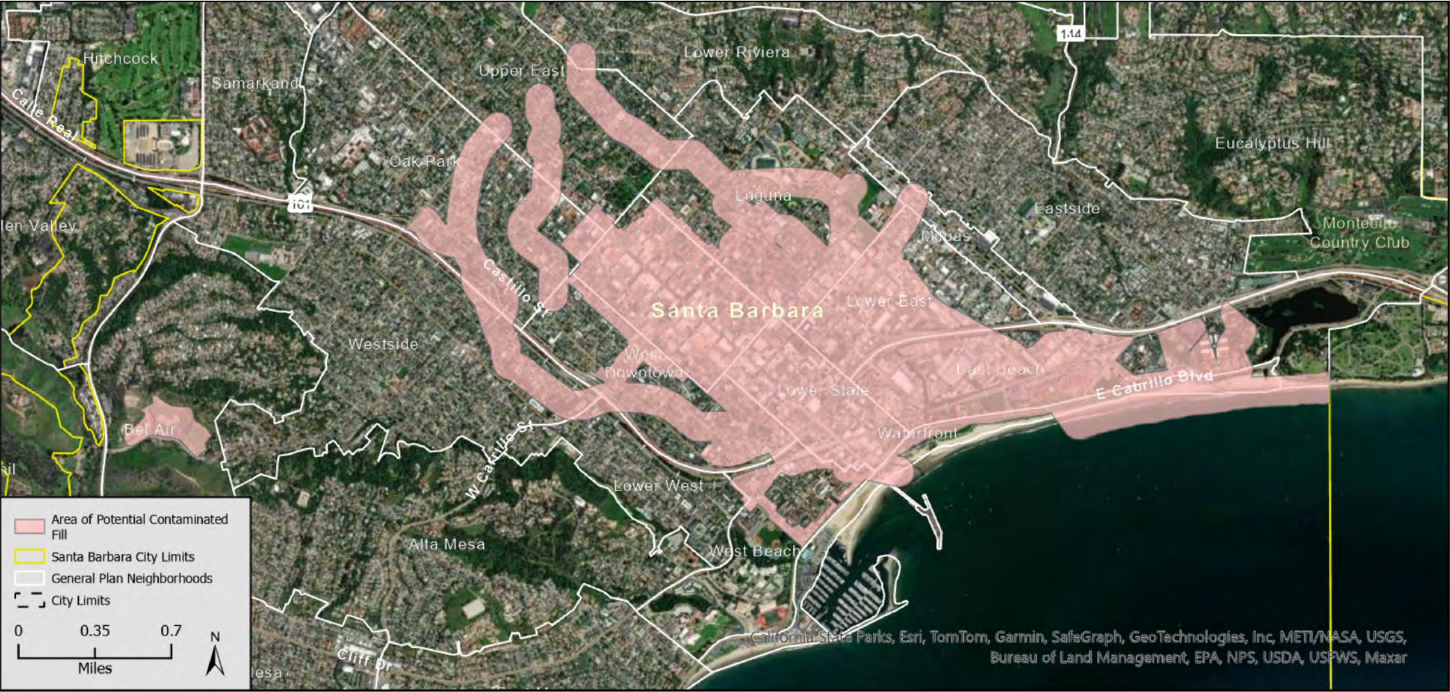
Figure 4.6-3 Areas of Potentially Contaminated Fill
