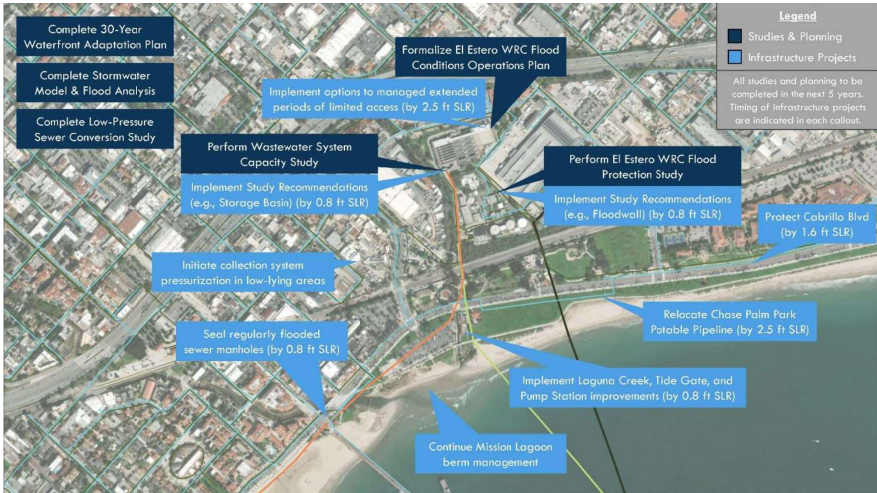
Figure ES-7. Adaptation Measures for Highest Near-Term and Mid-Term Infrastructure Risks from Climate Change
