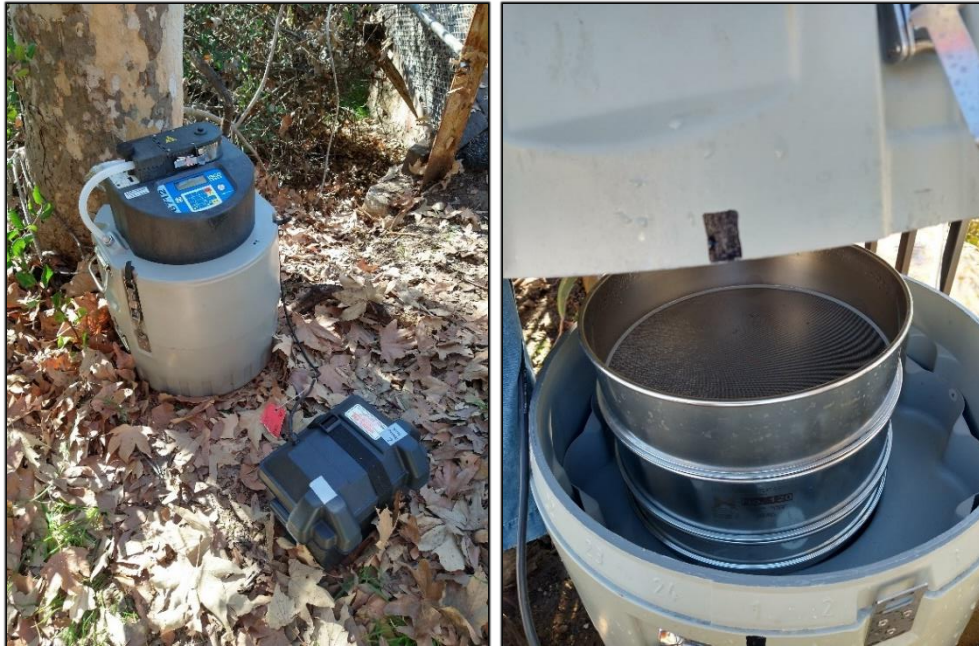
Figure 10: ISCO 6712 portable samples were modified and used for in situ microplastics filtration.
