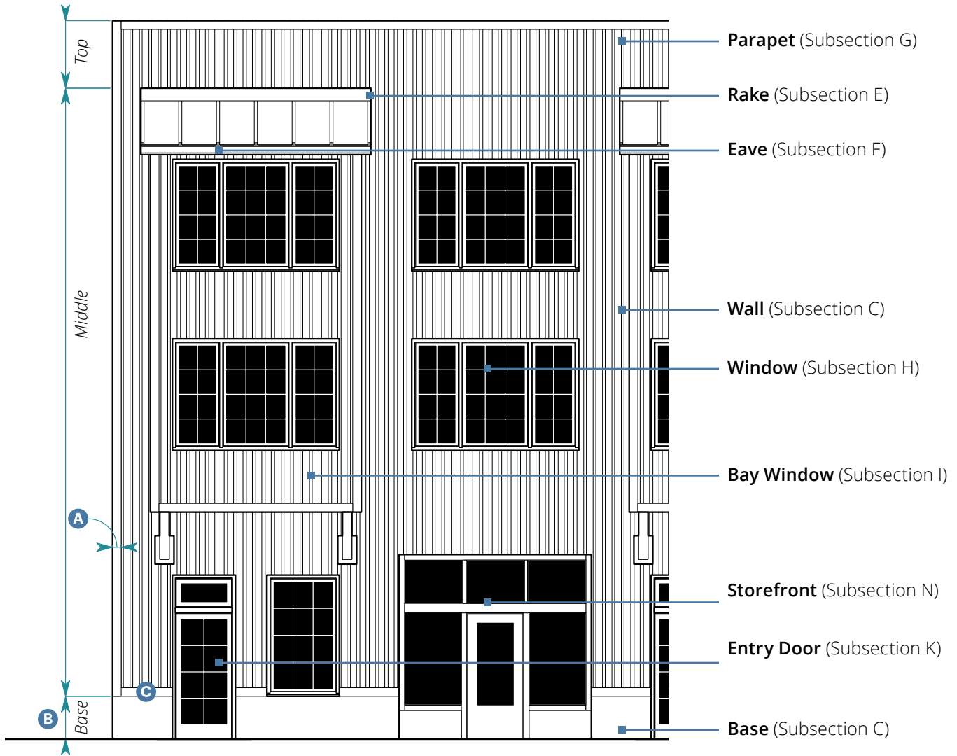
Example Building Elevation: Industrial
