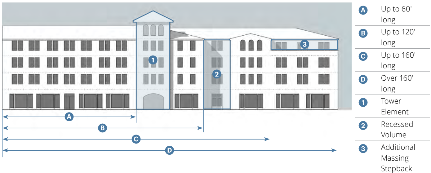
Figure 25.04.160.5: Example of Massing Features by Elevation Length
