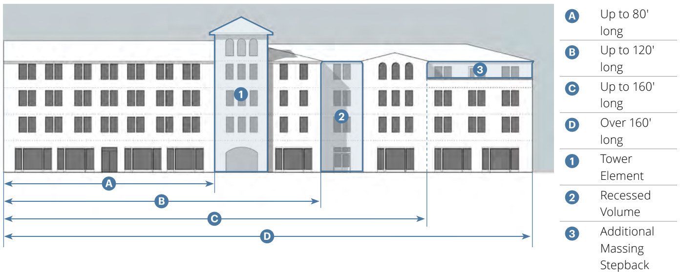
Figure 25.04.160.5: Example of Massing Features by Elevation Length
