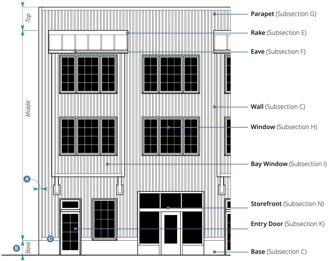
Example Building Elevation: Industrial
