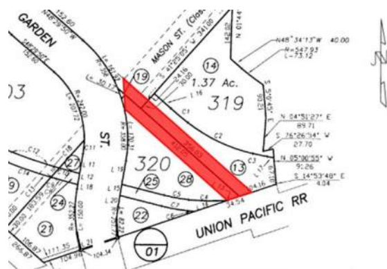
Figure 3 – Sewer Easement (Not To Scale)
