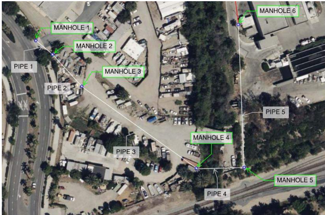
Figure 4 - Pipeline and Manhole IDs
