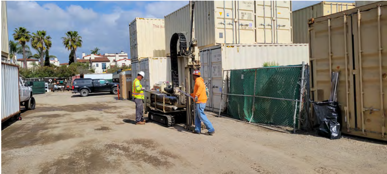
Photo 3. Geoprobe soil sampling at location SB7.
