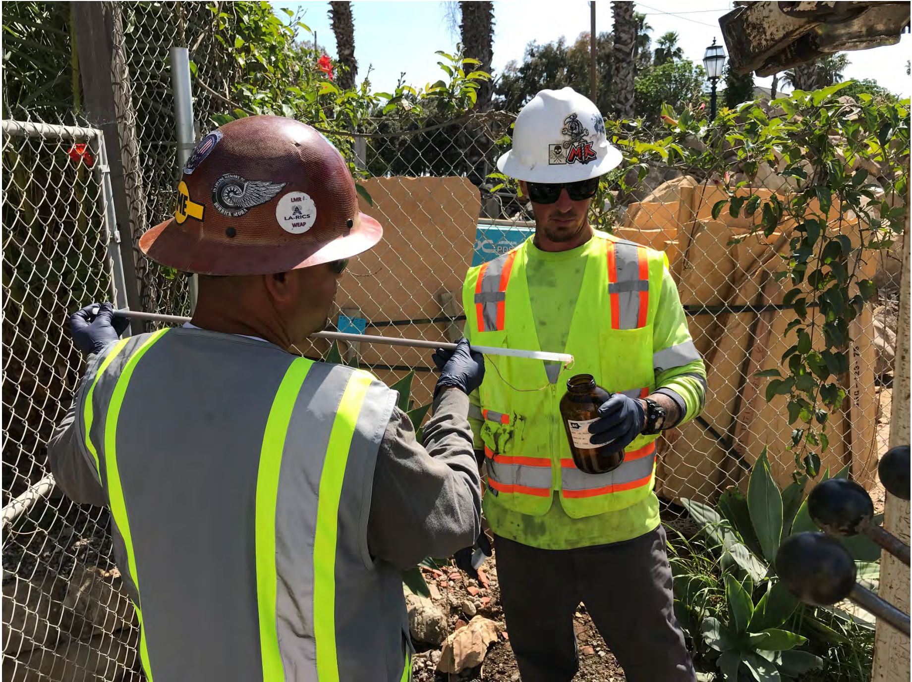
Groundwater sampling for TPH extractables SB18
