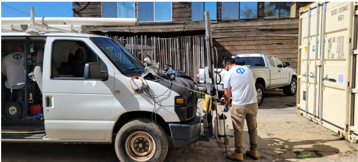
Photo 11. Soil vapor sampling at location SV3.
