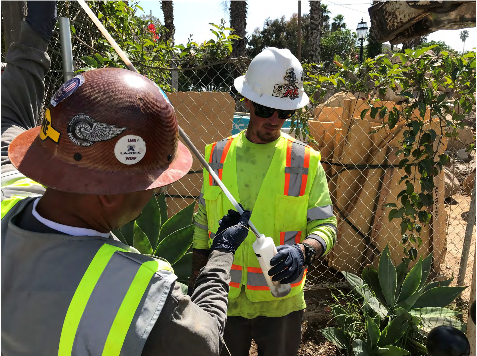
Groundwater sampling for metals, sample will be filtered in the lab SB18
