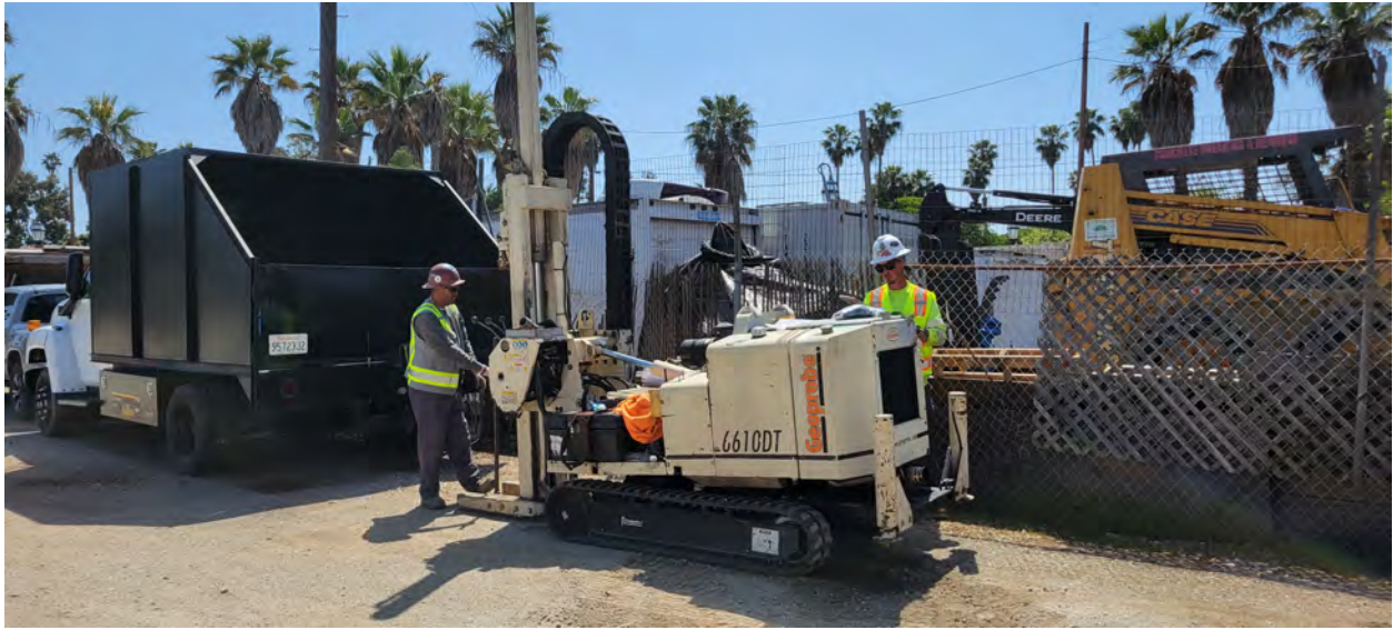
Photo 7. Geoprobe soil sampling at location SB20.
