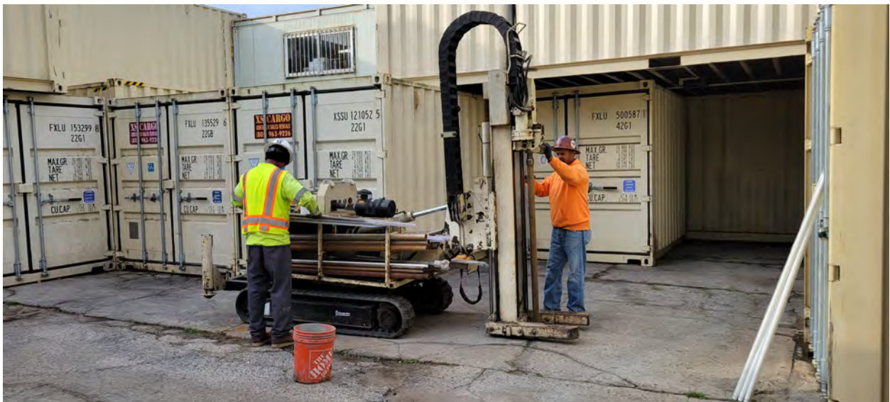
Photo 2. Geoprobe soil sampling at location SB3.
