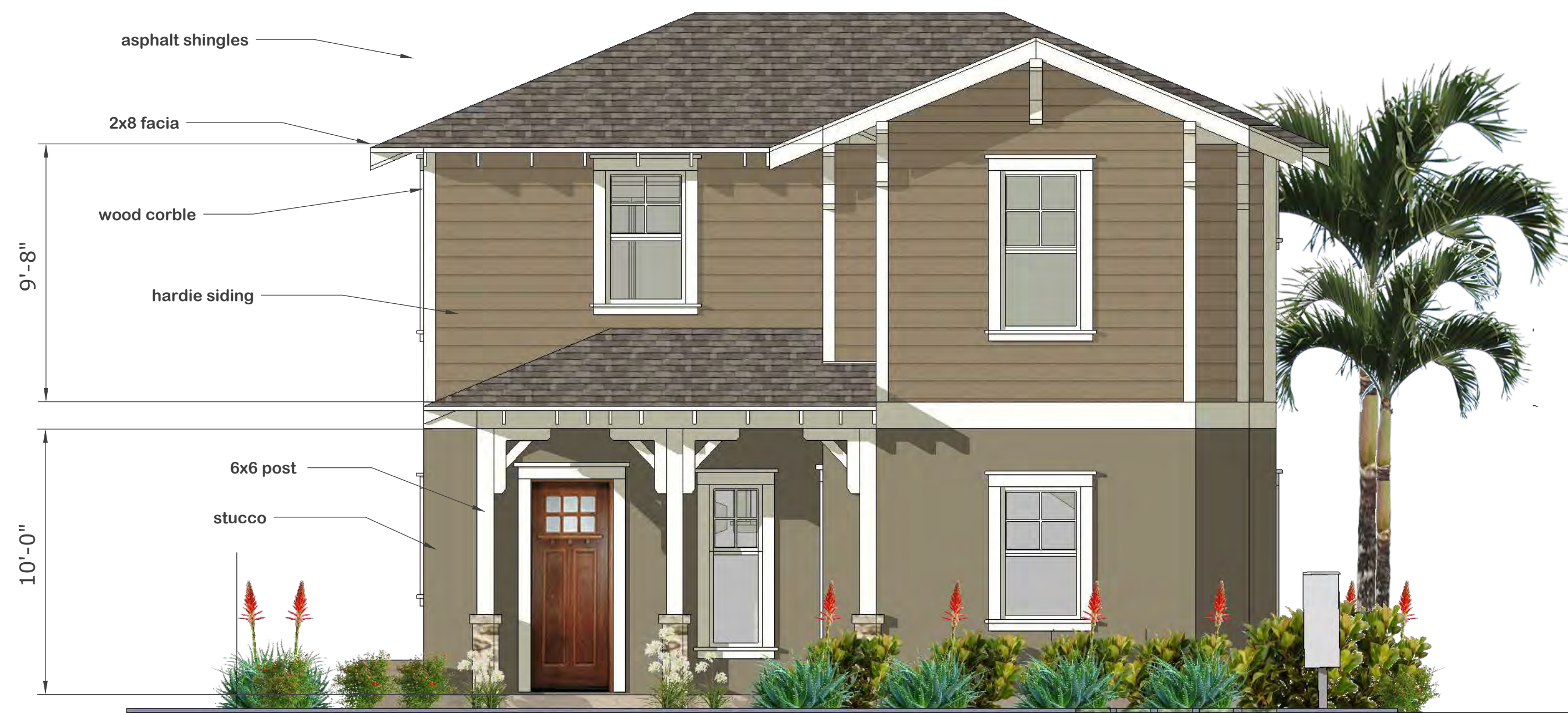
FRONT ELEVATION SCALE 1/8" = 1'-0"
