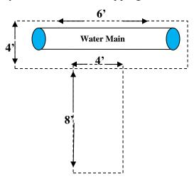
After traffic control and excavation are ready, the contractor will notify the Water Division Lead Operator and Public Works Inspector, who are assigned to the project. Call for inspection at least 24 hours before tap is scheduled, so that the trench can be inspected and given approval. (See **Public Works Inspection** Step 2 below)
