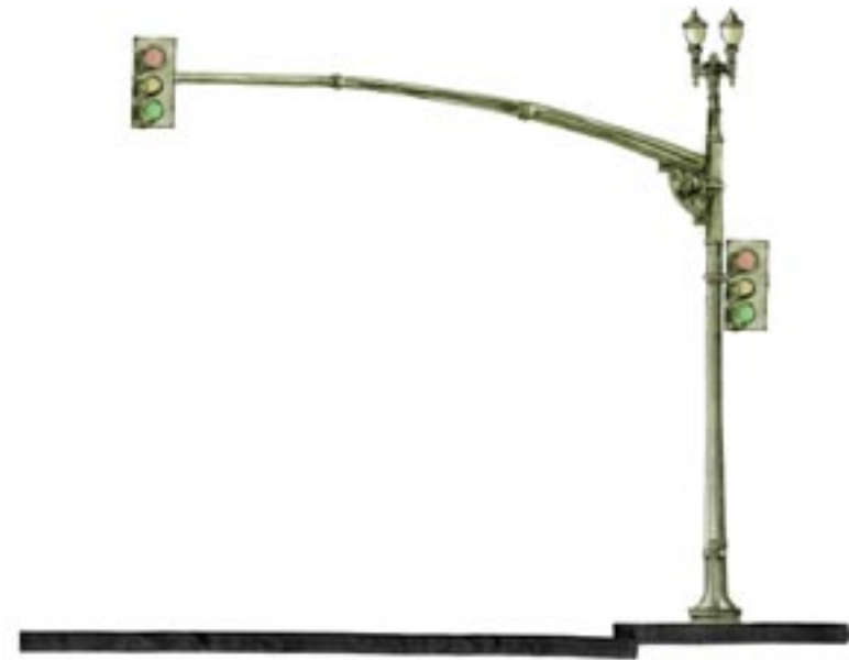
Typical Chapala Street Traffic Signal Elevation
