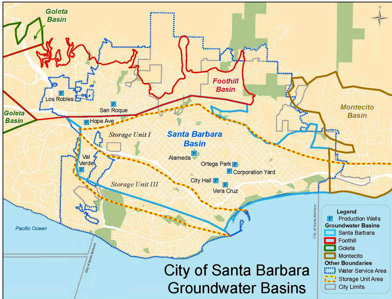
Figure 7: Groundwater Basins and Well Locations
