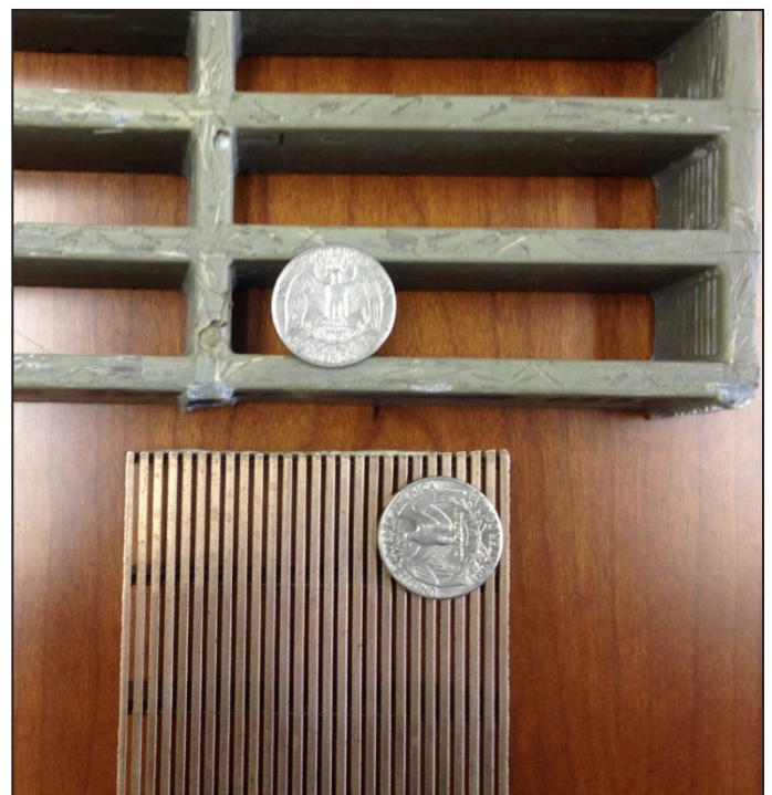
1990s era old intake screen (top) versus new intake screen (bottom)
